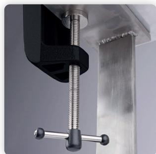
The SPANNFIX 9-205 ESD with dissipative powder coating is suitable for workbenches or work areas with a maximum table top thickness of up to 80 mm. The small vice with ball joint is quick and easy to attach to any workbench or table top due to its table clamp. A small pressure of the lever is sufficient and the clamped workpiece can be fixed steplessly and in any practical working position.
