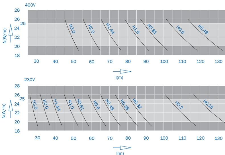
$$\text{Heating capacity Watt/m: } N' = \frac{U^2}{R \cdot L^2}$$
