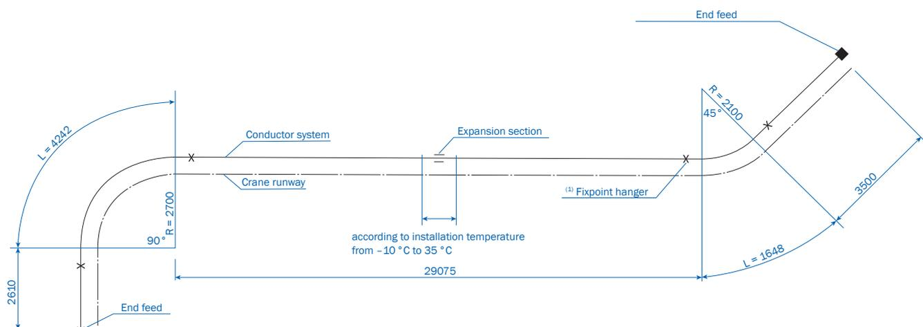
(1) Rest of conductor system to be installed with sliding hangers
