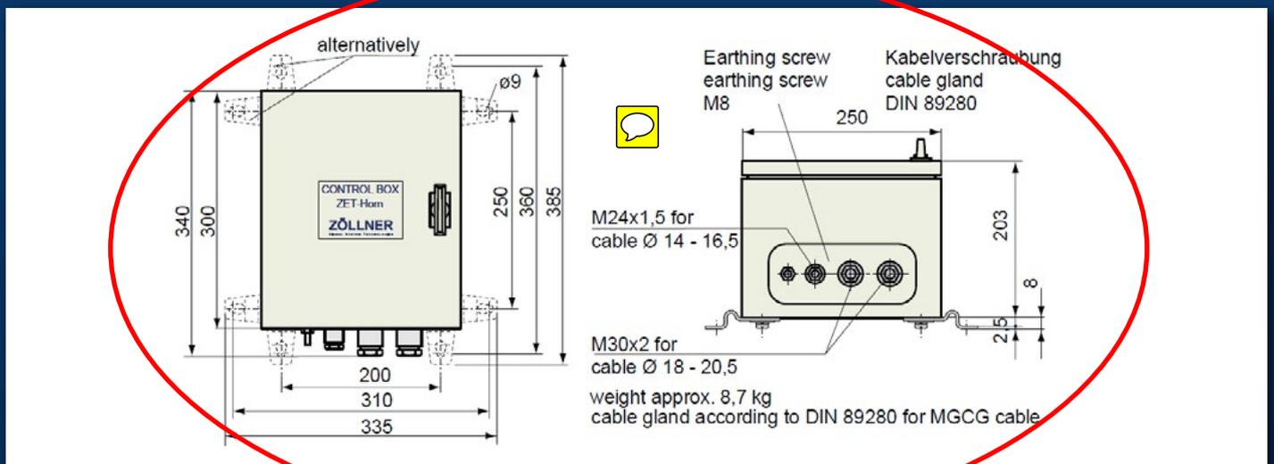
Standard control box (supply voltage 380 / 440 V - control voltage 115 / 220 V) - other voltages on request
