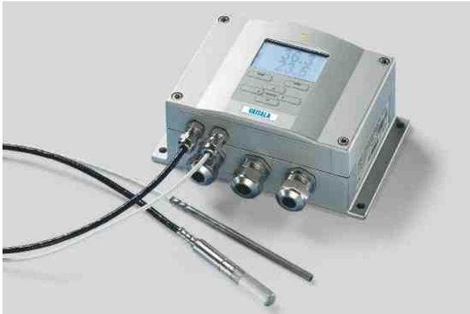
The HMT337 is ideal for the most demanding process and meteorological measurements in high-humidity condensing environments.
