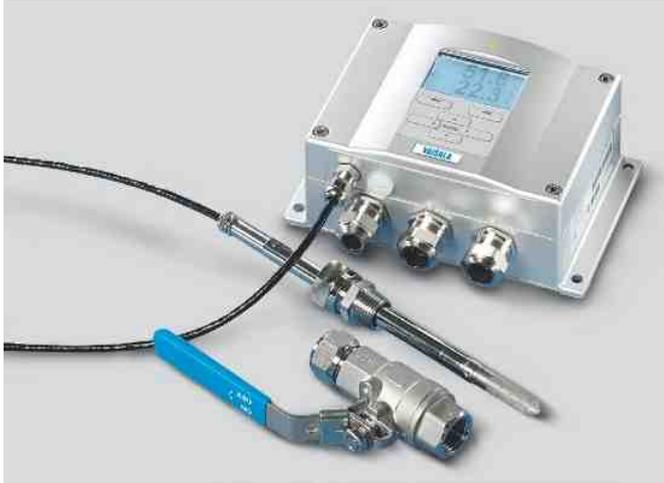
*The HMT338 is ideal for installations in pressurized processes where the probe needs to be removed while the process is running.*
