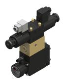
Basically the valve position indicator is a precision gear motor with a display indicating the flow of a certain oil volume through the unit. The gear wheels rotate according to flow and flow direction of the fluid. A built-in mini gear box with a gear ratio chosen
