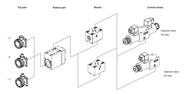
The VPI always consists of a VPI top part, a VPI bottom part and a VPI compensator block (TC or PTC).
