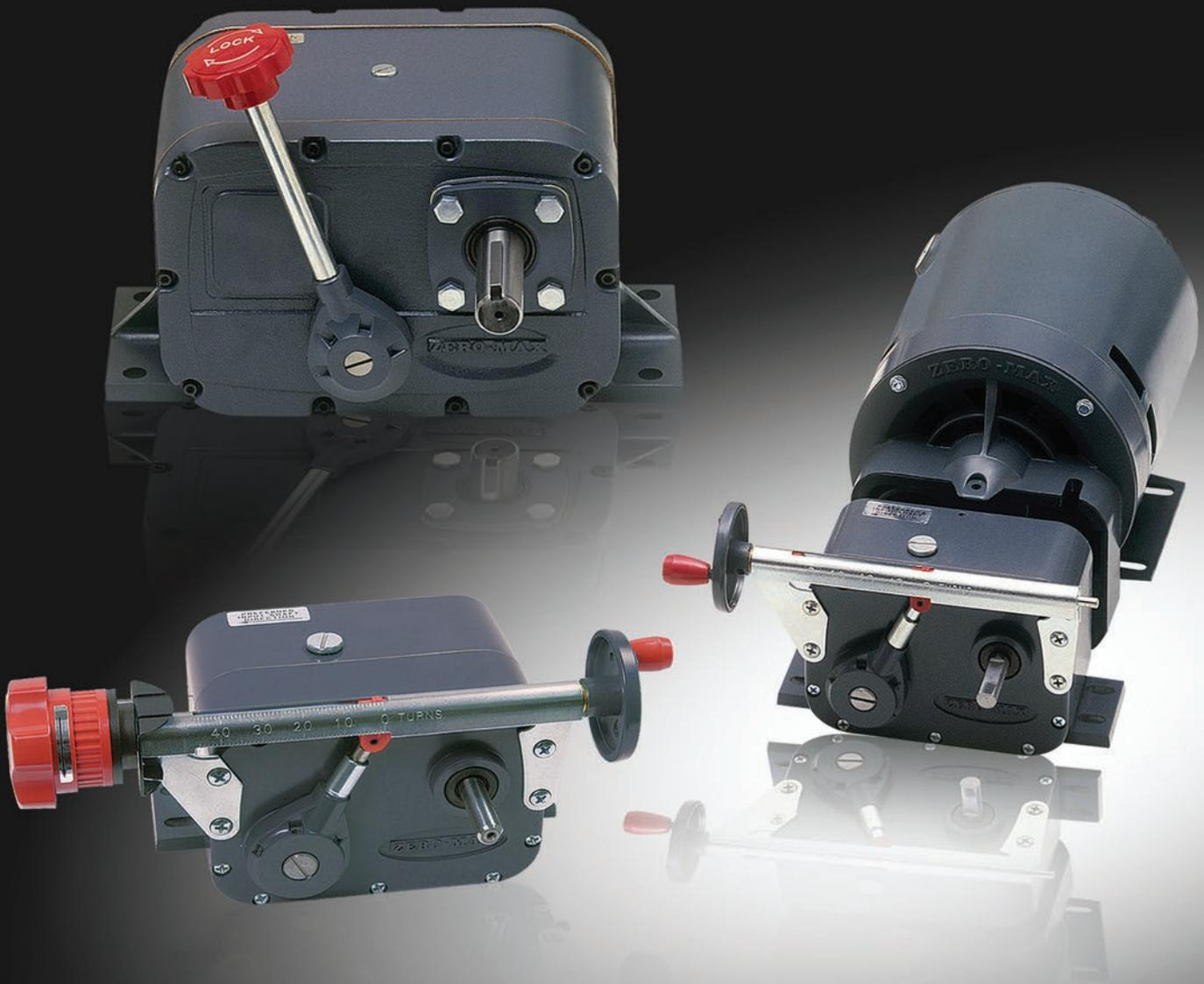
A Zero-Max Drive is a mechanical adjustable speed drive. Five sizes provide constant torque of 12 to 200 inch pounds throughout the speed range. The speed range is infinitely variable from 0 to 1/4 of the input speed under full rated load. This is generally stated as 0-400 RPM assuming an input of 1800 RPM.
