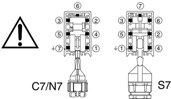
Trolley type S7 has different cable numbering.
