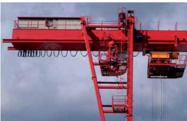
Our festoon systems offer the most flexible solutions for transporting flat or round cables and hoses. A wide variety of profiles and components guarantees reliable installations, adapted to the environment.
