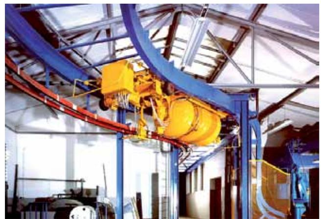
*Feed and control of a concrete skipper*
